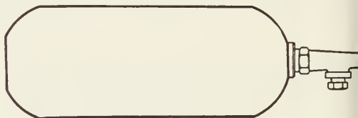
2-41. A refrigerant service cylinder. The color code for cylinder colors is as follows: Silver and black—sulphur dioxide, Orange and black—methyl chloride, Red and black—iso-butane, Yellow and silver—Freon —12.
